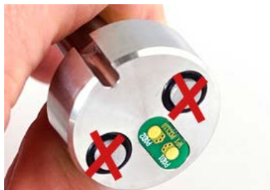
1a. Remove sinter filter. Do not re-use!
