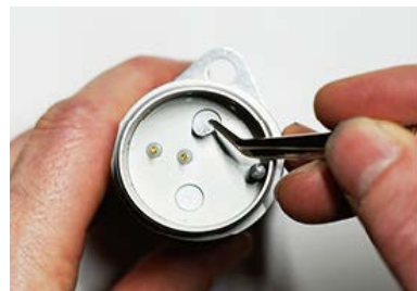
1b. Remove filter (new style) and dispose properly
