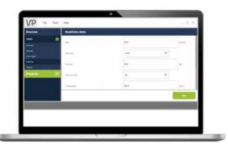
set via the software. VPStudio can be installed on your PC and communicates via the JB5 interface kit with the VPFlowScope via your PC's USB port.
