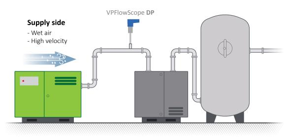
The VPFlowScope DP is preferably installed in the second horizontal piping after the compressor where there is less possibility for excess water. A cyclone separator is recommended upstream of the flow meter, to remove excess water from the system.
