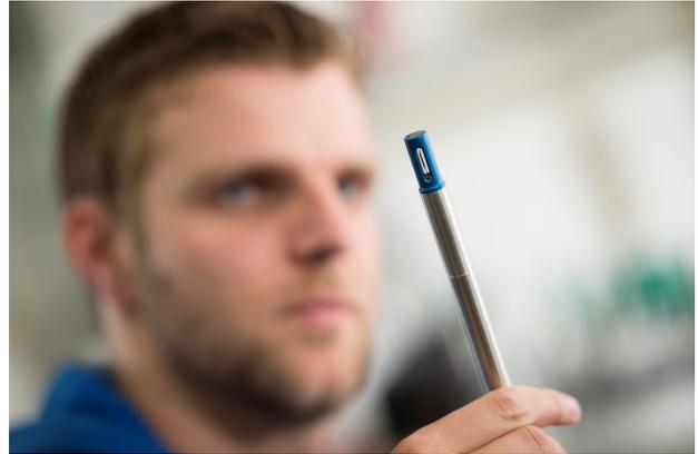
Periodical cleaning: Any dirt and oil in your air or gas can remain on the sensor. Cleaning the sensor may result in more accurate readings and a longer high performance of your device. Cleaning is a delicate procedure, so carefully check the instructions for your specific device.
